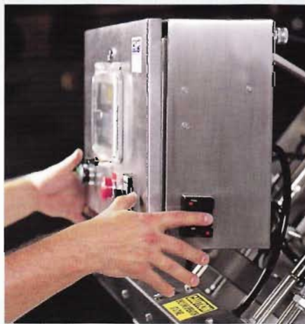
Dual optic-touch start switch adds safety and reduces carpal stress for the operator.
