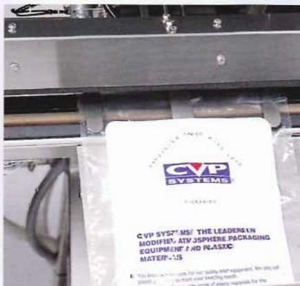
Bag stretchers minimize bag wrinkles for optimum seal integrity and aesthetics.
