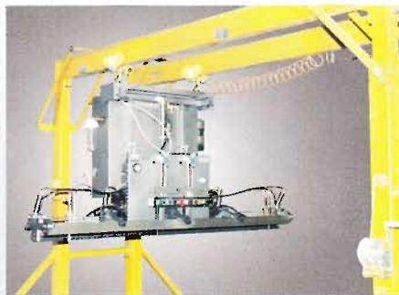
The A-200 Overhead can be mounted on an I-beam system for easy maneuverability over various bulk bin containers.
