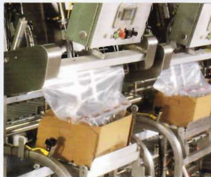
Head height can be adjusted for varying package sizes.
